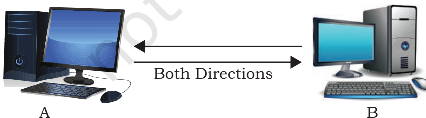
Figure 11.5: Full duplex transmission of data
