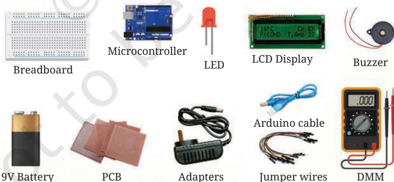
Figure 4.3: Electrical and electronic components
