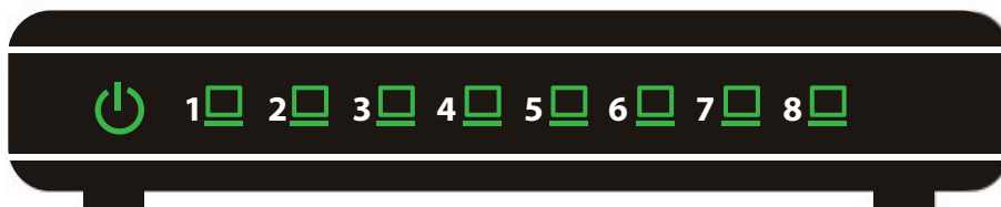
Figure 5.8: A network hub with 8 ports
